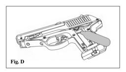
**WARNING:** Make sure your pistol is unloaded before removing or inserting the CO<sub>2</sub> cylinder to avoid accidental discharge and injury.
